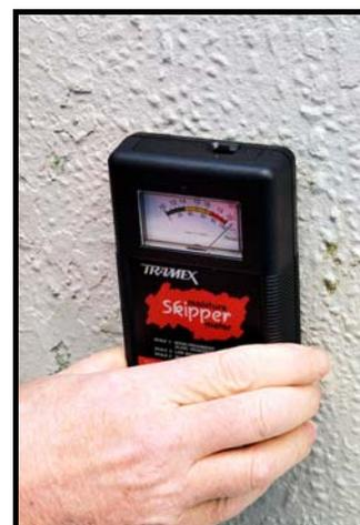
The purpose of this document, therefore, is to provide practical guidance on how to use the Tramex Skipper and Skipper *Plus* meters on conventional glass reinforced polyester (GRP) boat hulls. For a more detailed explanation please refer to the authors [Short Guide to Osmosis and its Treatment](#).
