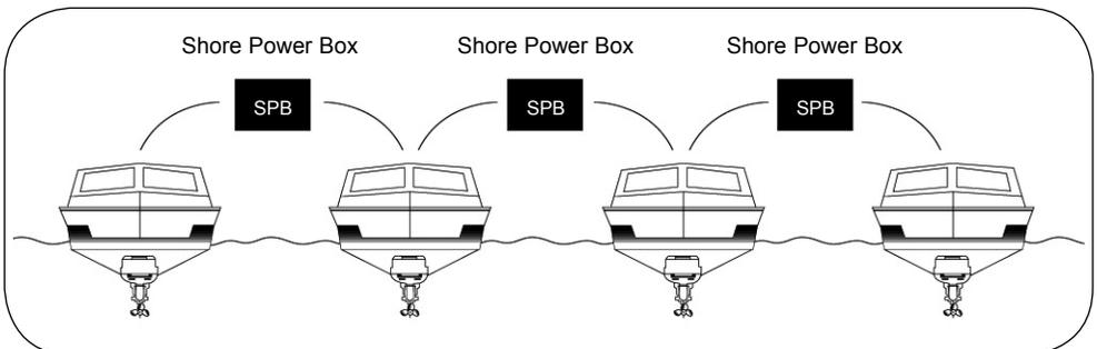
This earth cable is essential for our safety and also ensures correct operation of the shore power and vessels fuses and electrical trips: It is vital that this earth connection remains in circuit at all times: Removal can be fatal! In the event of a major electrical defect, lack of proper earth connections can be lethal to not only yourselves but to your immediate neighbours and even swimmers near the vessel!
