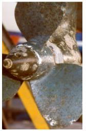
However, anodes will not prevent corrosion caused by poor choice of materials. This aluminium alloy drive leg and propeller was badly damaged by painting with copper based antifouling.
