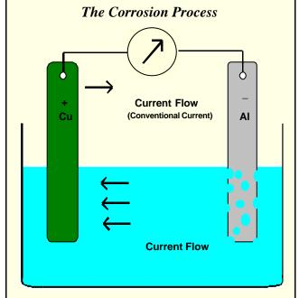
A typical corrosion cell showing how the negative electrode (or anode) is eroded, while the positive electrode (or cathode) remains free from corrosion.
