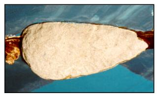
If they're working properly, anodes should last for two full seasons. When lifted, they should appear clean and lightly sandblasted without any deep pitting.
