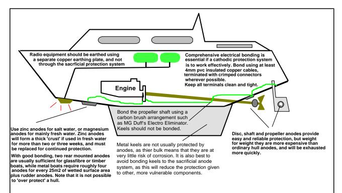
Correct installation of a Cathodic protection system. Note that all metal surfaces must be within 'line of sight' of an anode if they are to be adequately protected.
