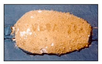
Correct choice of anodes is essential if you want optimum protection for your hull. Zinc anodes are not sufficiently active for long term use in fresh water, and will quickly form a thick crust which prevents them from working properly. Magnesium anodes work well in fresh water, but have a rather limited life in the briny.
