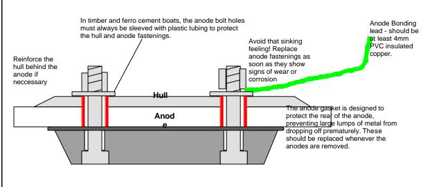
the need for bonding, although weight for weight these are rather more expensive than the larger hull anodes, and their lifespan is correspondingly shorter. Don't rely on bonding through the engine and gearbox though, as lubricating oil forms an insulating film on gears and bearings when they are turning.
