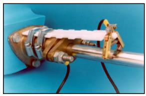
The MG Duff Electro Eliminator is a carbon brush arrangement, designed to ensure electrical continuity between your hull anodes, and propeller shaft.
